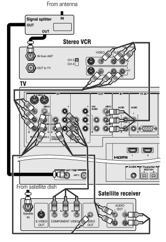
**Note:** The VIDEO/AUDIO OUT terminals output signals from the ANT 1, ANT 2, VIDEO 1, VIDEO 2, and VIDEO 3 terminals when the appropriate input mode is selected.
